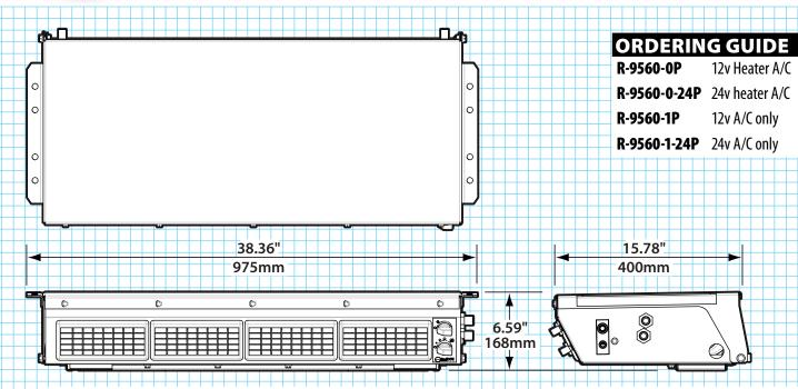
Instead of pulling air from the rear, the unit draws air from the bottom, which allows efficient airflow even when it's mounted near a back wall or some other tight location
